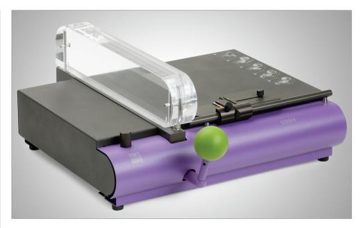
The Scoring Machine is designed to work hand-in-hand with the Fastback® 15xs to score card stock for covers that look good and open easily. The Scoring Machine can score card stock up to 20 points thick (.020" or .50mm). The patented Centering Guide eliminates any guesswork as to where to place the scores. No make-ready is ever needed. Place the bound book between the Book Thickness Rings and adjust the width to match. The Scoring Machine is now ready to produce perfect scores every time.
